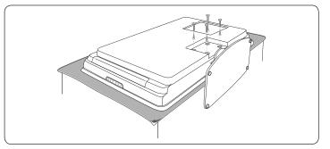
3. Firmly pull the stand from the bottom of the TV, being careful because the stand is heavy. Place both the stand and screws in a secure location for future reinstallation.
